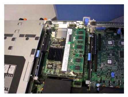
7. The next photo shows the Dell 2950 top cover off with PERC 5/E external RAID inserted.
